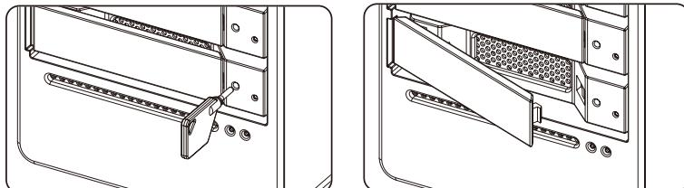
Step 4 Mount your hard drives onto the removable drive tray and secure it with the screws included in the accessory kit to avoid any damage to the hard drive due to accidental movements.
