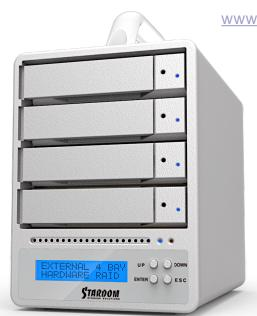
The SOHORAID SR4-SB3 is a four drive storage system with JBOD / RAID 5 / RAID 0 storage option for storing contents in large scales. Industrially designed with aluminum exterior that's built tough and durable for hard drive protection of the highest grade.
